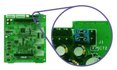
Refer to the following tables for the jumper settings and the appropriate ID# for each SCSI HDD bay.
